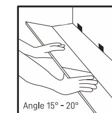
Assemble the second row on the subfloor, tilt and push to attach to the first row, then click into place.
