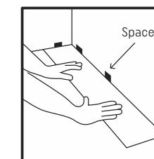
Start at a corner, tongue side facing wall, with spacers for an 8-12 mm expansion gap.
