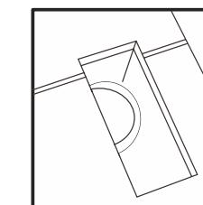
For heating vents, cut the plank to length, measure and mark areas to cut out, then cut allowing for expansion.
