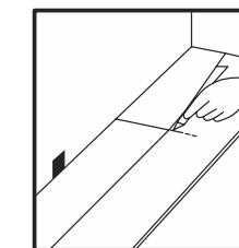
For the last plank of a row, measure, mark, score, and snap off the required length, then insert.
